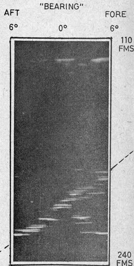
FIGURE 5. Record obtained with 3-beam echo-sounder. (Courtesy, Institute of Navigation.)
