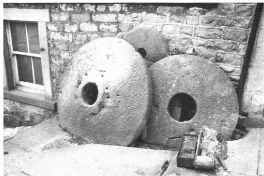
Plate 8 Grit millstones at Conder Mill, Lancs. The two larger ones are 5 ft 7 in and 4 ft 6 in diameter respectively. These stones are thought to have been made from local rock in the Quernmore area.
