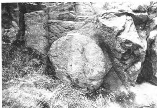
Plate 2 Partially-cut millstone still attached to main body of rock at Mow Cop, Cheshire. 4 ft 8 in diameter (white bar is 12 in long); centre-pop visible.
