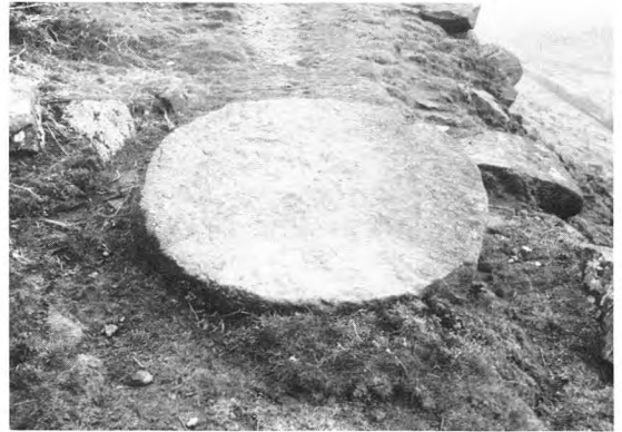
Plate 5 Circular block of millstone grit prepared as blank for millstone on Curbar Edge (at about SK 258750); 56in diameter, 10in thick at cylindrical edges, no hole yet cut.
