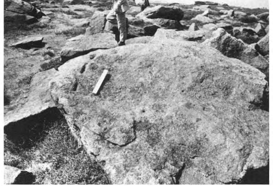
Plate 3 Block of millstone grit on Hathersage Moor (at SK 251807) evidently intended as blank for a millstone. Centre 'pop' visible, 34in from the three wedge marks, thus indicating intended finished diameter of about 64in.
