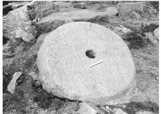
Plate 7 Millstone partially formed from daystone on Hathersage Moor (at SK 255805), flat face cut and edges partly cut, 68in diameter, 8in hole cut a few inches deep, not yet turned over for convex surface to be shaped. Total thickness of blank did not exceed 12in, so degree of convexity would have had to be small.
