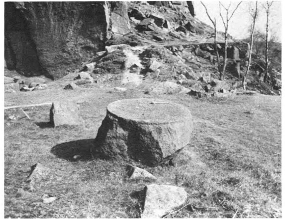
Plate 15 Block of millstone grit at small Bole Hill quarry (at SK 249799) with flat face and circular shape cut, 36in diameter. Probably twentieth century.
