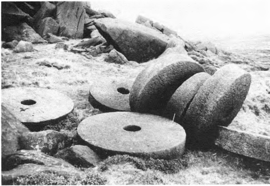
Plate 14 Group of completed millstones at Stanage Edge (at about SK 252830). Probably early twentieth century. Dimensions: 1 stone 49in diam, hole 9in diam, 12½in thick at edge: 1 stone 56in diam, hole 11 in diam, 14in thick at centre, 12in thick at edge: 4 stones 60in diam, hole 11in diam, 15in thick at centre, 12½in thick at edge: 1 stone 61in diam, otherwise same as 4 stones above.
