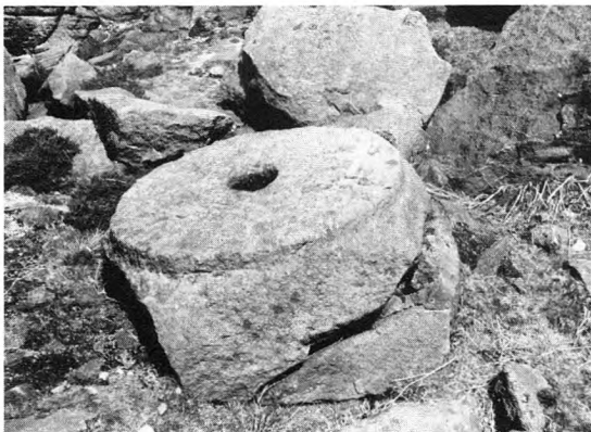
Plate 6 Daystone on Hathersage Moor (at SK 251807) partly worked as millstone, with flat face and circular shape cut, 46in diameter, 8in hole cut about 6in into stone.
