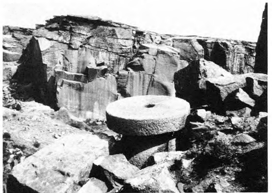
Plate 13 Finished cylindrical millstone at quarry on Wildmoorstones Edge (at SK 265810), 52in diameter. Probably twentieth century.
