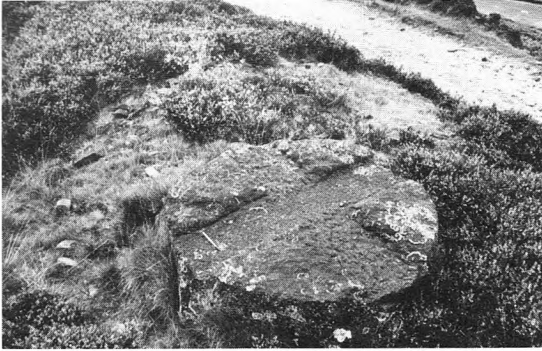
Plate 16 Stone cut roughly circular and with crossed grooves cut on plane of face, at Millstone Edge (at SK 248803). The presumption is that the crossed grooves represent the beginning of the face-dressing process, with the remainder of the face to be cut by a less-skilled worker. 60in diameter. Few other specimens like this have been found in the Peak District (only on Beeley Moor), but similar examples of the process have been found in Wales (see ref. 2).
