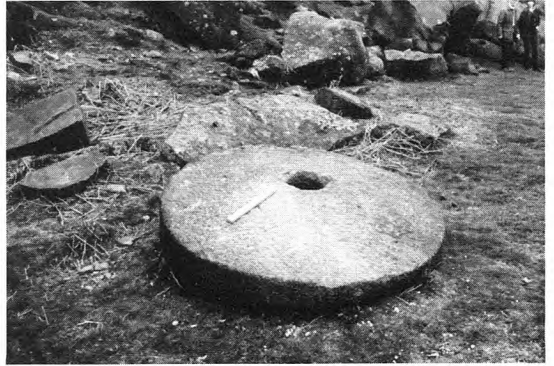
Plate 11 Completely finished and apparently undamaged intermediate-type millstone at Curbar Edge (at about SK 258750), 58in diameter, hole 8in diameter, thickness 14in in hole, 9in at edge, cylindrical in form. (White bar is 12in long.)
