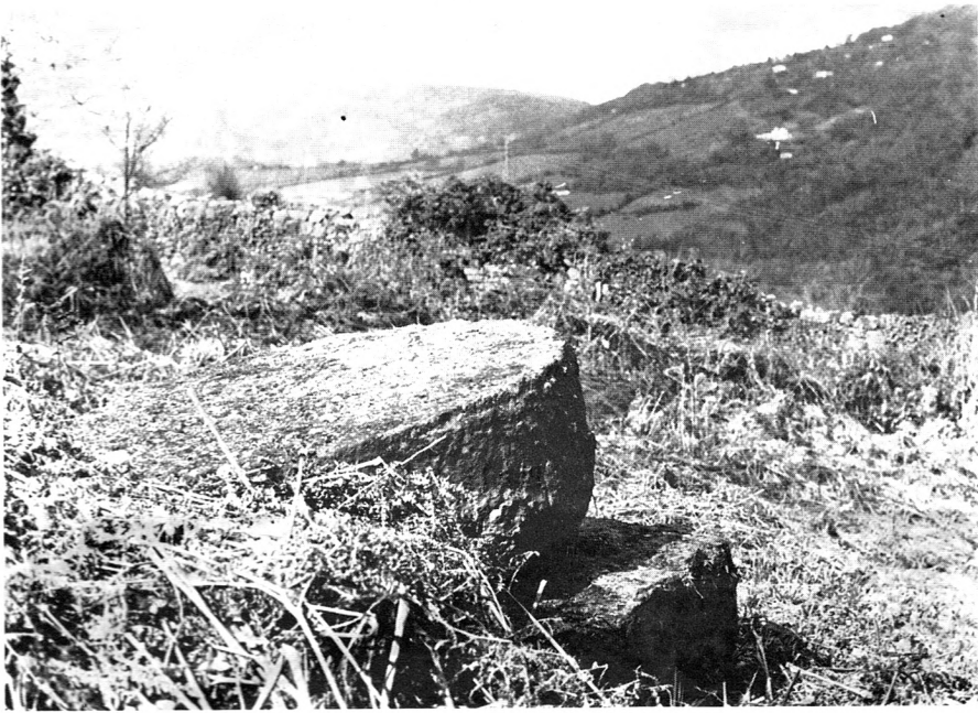
Conglomerate (Welsh) millstone, supported on piece of stone to raise it above the ground for finishing. Abandoned specimen at Penallt, Gwent.
