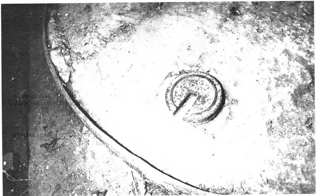
Balancing of French-burr stone by weight fixed in plaster backing.
