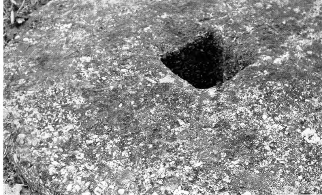
Page 321 (above) Close-up view of part of an abandoned cider-mill-stone (or 'runner') to show the nature and texture of the quartz conglomerate used for millstone making at Penallt; (below) a curious stone found in Quarry B at Penallt. The ruler laid on the stone is 1ft long See D. G. Tucker, 'Millstone Making', pp 229-39
