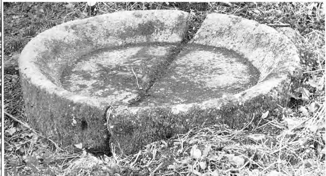
Page 322 (above) The runner in an old cider mill, belonging to Mr Downes of Penallt, which is still in working order; (below) base-stones (or 'chase') of a derelict cider mill at Penallt, showing the construction in two semicircular pieces See D. G. Tucker, 'Millstone Making', pp 229-39
