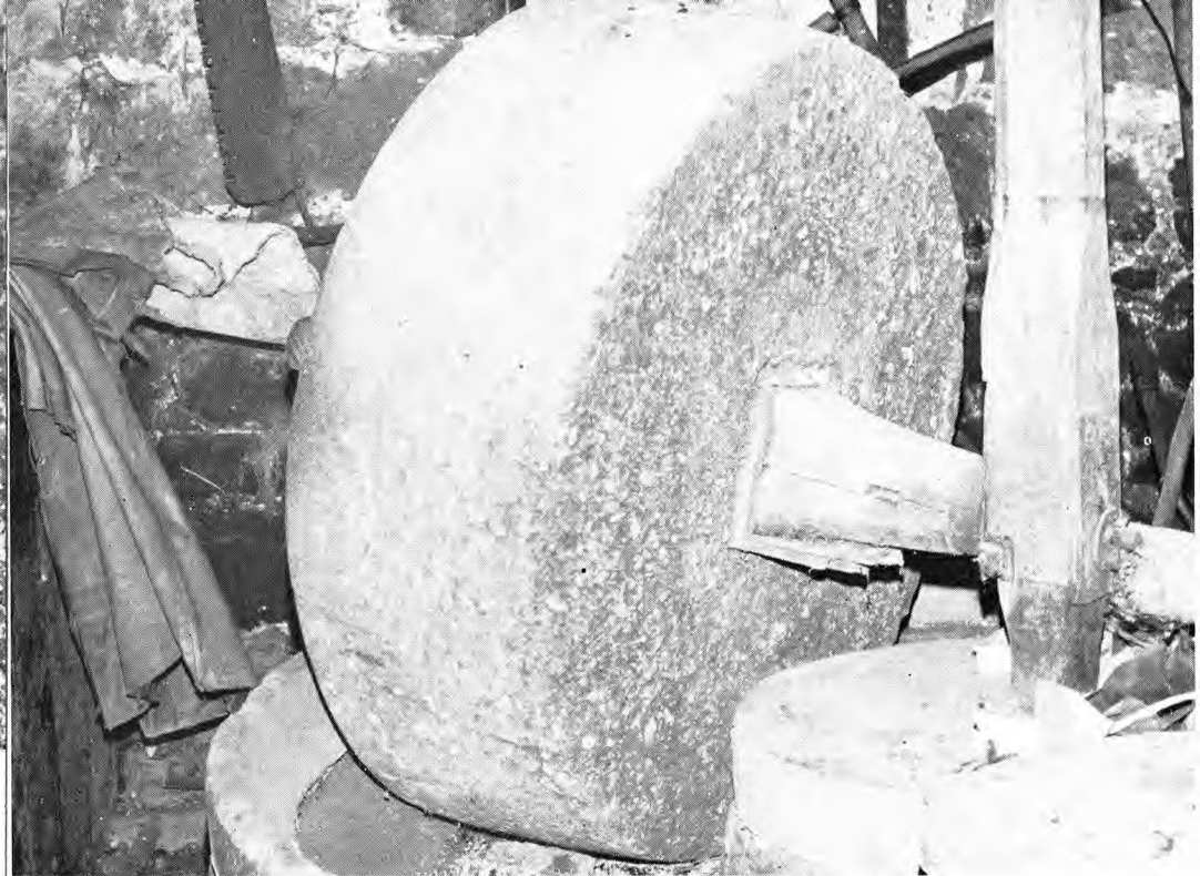
Page 322 (above) The runner in an old cider mill, belonging to Mr Downes of Penallt, which is still in working order; (below) base-stones (or 'chase') of a derelict cider mill at Penallt, showing the construction in two semicircular pieces See D. G. Tucker, 'Millstone Making', pp 229-39
