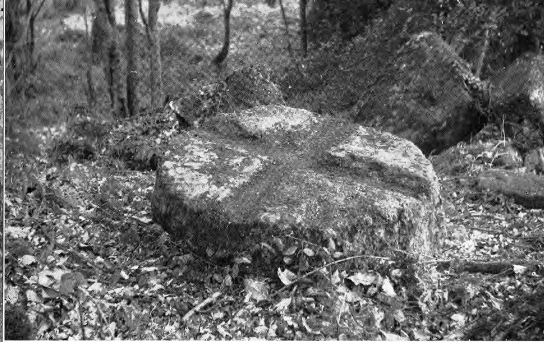
Page 324 (above) Abandoned unfinished stone at Quarry A at Penallt, showing the two crossed channels cut into the top, presumably as guides for the dressing of the whole surface; (below) abandoned unfinished stone (almost certainly for a cornmill) at Quarry E at Penallt See D. G. Tucker, 'Millstone Making', pp 229-39
