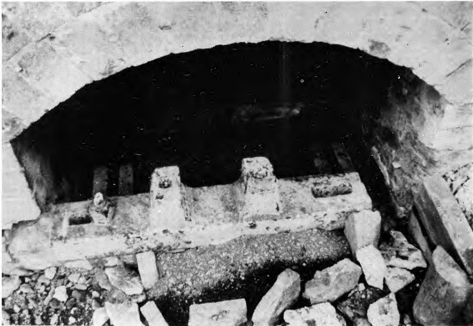
Plate 20. (below) Iron casting, with horns to carry the bearing for the iron axle.
