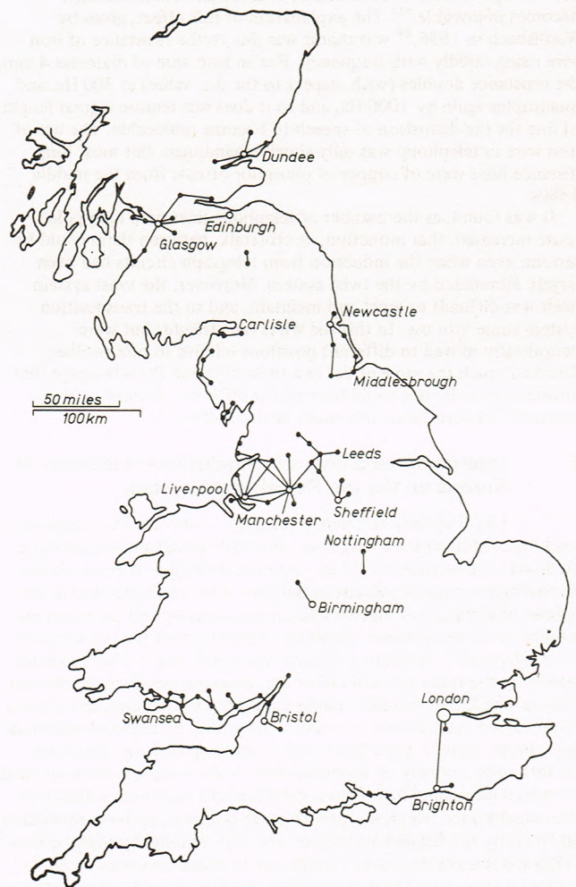
Fig. 3 Interurban telephone system in Britain in 1887
