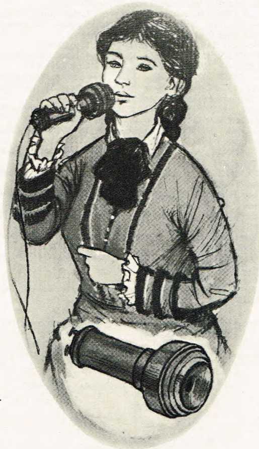
1 First commercial telephone set (1877). The customer did not have an earphone and microphone. There was one electromagnetic transducer in the instrument, so that the speaker had to make clear to his partner that he had finished speaking and was going to transfer the instrument from his mouth to his ear
